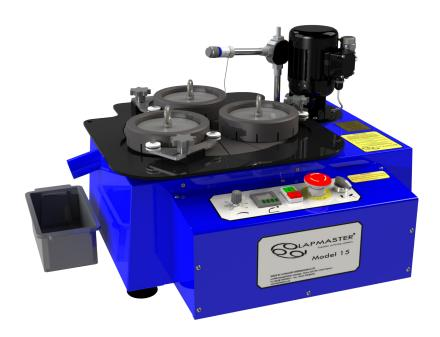
The Lapmaster Wolters Model 15 is a bench mounted unit with a heavy duty carbon steel weldment base.
